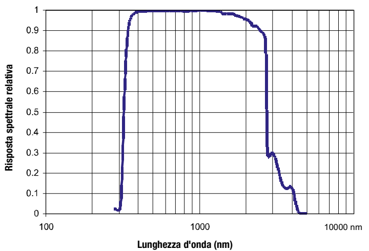
Figure 1. Typical spectral response of the pyranometers.
